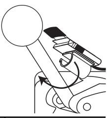
Position the Switch up towards the end of the draw-handle bar to complete the Installation.
