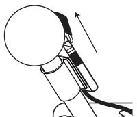
Be sure to fully engage the Spigot Switch jack to the Flavor Burst™ keypad jack for normal operation. Do not neglect to check this connection during daily startup.
