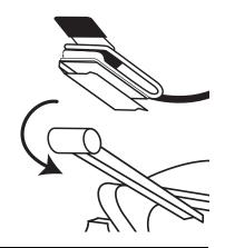
Position the Switch up towards the end of the draw-handle bar to complete the Installation.
