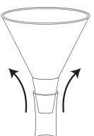
Run cold water over the area where the tube is attached to the funnel to set the connection.
