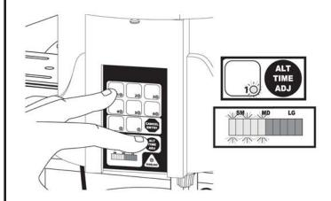
The number of lighted bars in the graph represent the length of time the serving is dispensed. Use the following chart to determine the bar graph setting needed for the desired serving size time.
