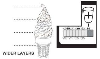
To decrease the timing (for more narrow layers), press the SMALL CUP (-) key until the correct number of bar graph lights are lit.
