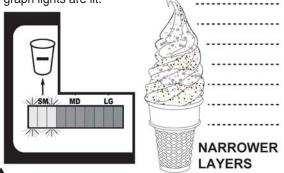
NOTE: IF THIS IS THE FIRST TIME ALTERNATING INGREDIENT TIMING HAS BEEN SET, SET THE TIMING TO ONE LIGHT (.5 SECONDS), DRAW A SERVING, AND THEN ADJUST THE TIMING FOR WIDER LAYERS IF NEEDED.
