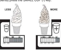
Repeat steps 2 and 3 to adjust for each flavor that needs to be adjusted for concentration.
