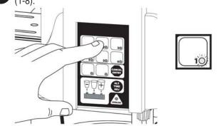
To increase the ingredient concentration (ie, add more ingredients to the serving), press the LARGE CUP (+) To decrease the concentration (ie, for less ingredients) press the SMALL CUP (-) key.
