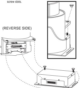
Position the mounting base assembly on top of the freezer. If the draw handle is operated by the left hand, the center of the mounting base should be mounted within 3" to the right of the draw handle. If the draw handle is operated by the right hand, the mounting base should be mounted within 3" to the left of the draw handle. Once in position, secure the mounting base to the CW 178C bracket using the screws provided.
