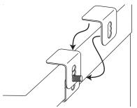
Slide the bracket assembly firmly together over the screws through the designated screw hole on each side bracket. Tighten the bracket assembly screws and install thumb nut onto each anchor bracket screw.
