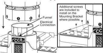
To clean the area under the Mounting Bracket, remove the carousel from the mounting base and rotate the assembly up and back over the reservoir cover. The assembly is hinged on the anchor brackets.
