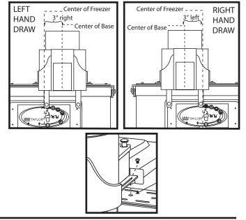
Ensure the chip hopper funnel is in place within the mounting base and install the carousel over the funnel with the #1 dispensing module in front. Ease the carousel down onto the mounting base until the electrical connection engages.
