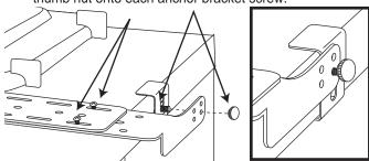
Install the mounting base onto the base extension and secure it with the thumb nut. Ensure the thumb nuts are totally seated in the recess of the mounting base
