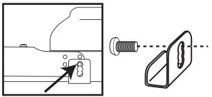
Slide the bracket assembly open and install the lower anchor bracket up under the lip of the freezer cap directly behind the appropriate side bracket screw hole. Repeat steps 4 and 5 to install the other anchor bracket on the other side of the freezer.
