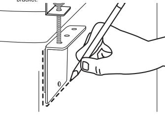
Disassemble the Mounting Bracket assembly. Remove the protective backing from the anchor brackets and press each one onto the freezer within the markings.
