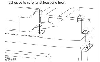
Install the mounting base to the mounting base extension and tighten the hand screws to secure. Adjust the vertical stabilizer bar thumb nuts to ensure the mounting base is level.
