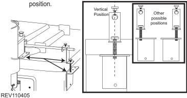
Using a soft lead pencil, mark around each anchor bracket.
