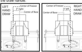
Adjust the vertical stabilizer bar screws to extend the bars downward as far as possible without obstructing any freezer operational controls. Tighten the screws to secure the position.
