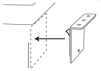
NOTE: IT IS HIGHLY RECOMMENDED SELF-TAP SCREWS ARE INSTALLED ON THE ANCHOR BRACKETS FOR MORE SECURE MOUNTING IF POSSIBLE. THE ADHESIVE TAPE IS NOT SUITABLE FOR PERMANENT OR LONG-TERM MOUNTING. IF SCREWS ARE NOT USED, FLAVOR BURST WILL NOT BE RESPONSIBLE FOR DAMAGE IF THE UNIT BECOMES DISCONNECTED FROM FREEZER.
