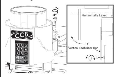
Ensure the chip hopper funnel is in place within the mounting base and install the carousel over the funnel with the #1 dispensing module in front. Ease the carousel down onto the mounting base until the
