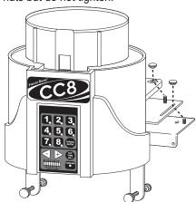
Set the assembly as far back on the ledge without obstructing any of the freezer operational controls. Slide the base and extension as far back onto the mounting bracket plate as possible and tighten the thumb nuts.
