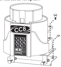
Set the assembly as far back on the ledge without obstructing any of the freezer operational controls. Slide the base and extension as far back onto the mounting bracket plate as possible and tighten the thumb nuts.
