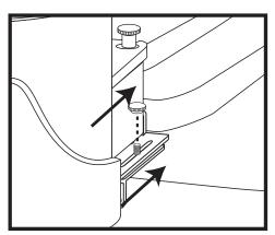
Thoroughly clean and dry the surfaces of the freezer where the mounting assembly will be attached. Using a soft lead pencil, mark the center of the freezer top, directly above the door spout.
