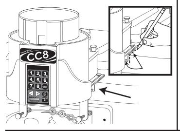
Remove the mounting bracket plate from the assembly, remove the protective tape from the adhesive, and press the bracket within the pencilled marks on the freezer. Carefully drill a 1/8" hole into the freezer through each of the screw holes.
