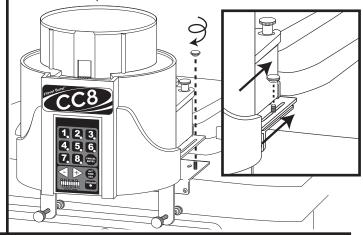
Adjust the vertical stabilizer bar thumb nuts to ensure the mounting base is level.
