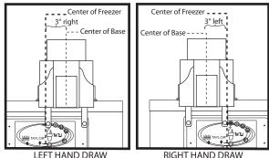
Use the vertical stabilizer bar screws to extend the bars downward as far as possible without obstructing any freezer operational controls. Tighten the screws to secure the position.
