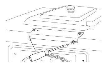
Remove the thumb nuts from the mounting plate. Install the mounting base and extension onto the freezer bracket plate, slide the base and extension as far back as allows and tighten the thumb nuts of the bracket plate to secure.
