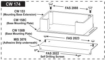
Assemble the mounting base to the mounting base extension and tighten the thumb screws to secure. Place the screw studs of the the mounting bracket plate within the extension plate grooves as shown. Attach the thumb nuts but do not tighten.
