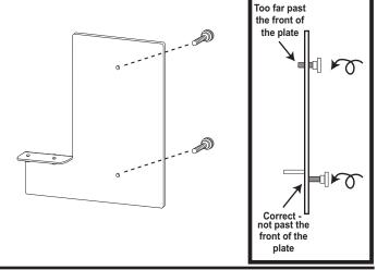
Using the two screws, attach the bracket to either set of screw holes on underside of the Mounting Base.
