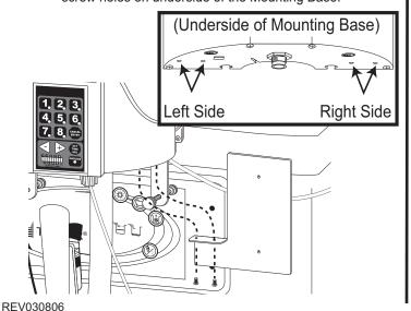
Slide the Keypad onto the bracket. Tighten the hand screws from the back side of the bracket to secure the Keypad.
