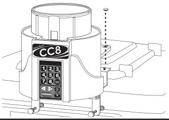
Adjust the vertical stabilizer bar thumb nuts to ensure the mounting base is level.
