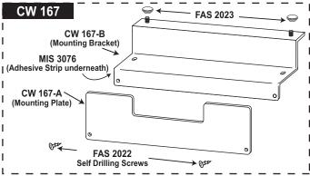
Assemble the mounting base to the base mounting bracket and tighten the thumb nuts to secure.
