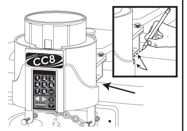
Remove the mounting bracket plate from the assembly, remove the protective tape from the adhesive, and press the bracket within the pencilled marks on the freezer. Carefully drill a 1/8" hole into the freezer through each of the screw holes.
