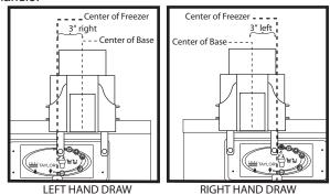
Use the vertical stabilizer bar screws to extend the bars downward as far as possible without obstructing any freezer operational controls. Tighten the screws to secure the position.
