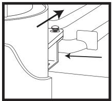
Thoroughly clean and dry the surfaces of the freezer where the mounting assembly will be attached. Using a soft lead pencil, mark the center of the freezer top, directly above the door spout.
