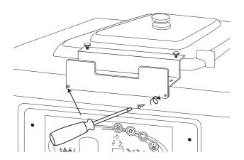
Premove the thumb nuts from the mounting bracket. Install the mounting base onto the mounting bracket studs and install the thumb nuts of the bracket plate to secure.
