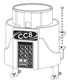
Set the assembly as far back on the ledge without obstructing any of the freezer operational controls. Slide the base and extension as far back onto the freezer as possible.
