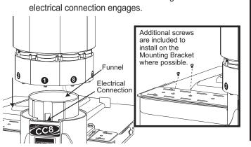
the mounting base to the CW 163 plate posts using the hand knobs.
