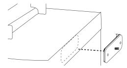
Loosen the screws on one end of the bracket assembly and slide the bracket assembly wide enough to install it over the anchor brackets. Once installed, slide the bracket assembly firmly together over the anchor bracket posts and tighten the screws. Install and tighten the hand nuts.
