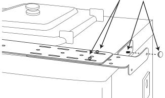
THE CW 163-A KIT REPLACES THE BASE EXTENSION AND MOUNTING SCREWS OF THE CW 178 BRACKET ASSEMBLY.
