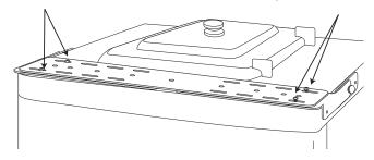
Position the mounting bracket so that it is as close to the reservoir cover as possible without having the front edge of the bracket assembly back beyond the front edge of the freezer. Using a soft lead pencil, mark around both anchor brackets.
