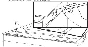
Pinch the primer ampule at the dot on the tube to release the primer fluid into the brush end. Apply the primer to the areas where the anchor brackets will be attached. Allow the primer to dry completely before proceeding (approximately 2 minutes).
