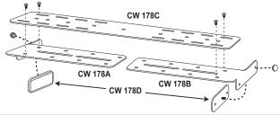
2 Ensure the freezer reservoir cover is in place. Place the assembled bracket on top of the freezer front and adjust the width of the bracket so that the anchor brackets are snugly pressed against the side of the freezer. Tighten the bracket screws to secure the assembly.
