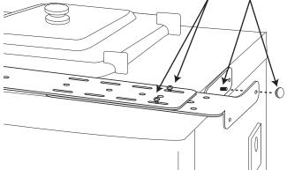
The mounting base can be mounted to either side of the freezer. The CW 163 plate will line up with only one set of screw holes on each side of the central mounting bracket plate. If the draw handle is operated by the right hand, the mounting base should be installed in the left side set of screw holes. If it is operated by the left hand, mount the assembly on the right. Once in position, secure the plate to the CW 178C bracket using the screws provided.
