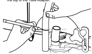
Remove the Hopper Tube Assembly and cut the tube 3/4" longer than where the tube was marked.
