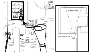
Holding up the Hopper Tube Assembly as far as it will go into the Mounting Base, mark where the tube lines up with the top of the Tube Adapter.
