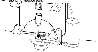
2 Insert the top of the Hopper Tube Assembly into the opening of the Mounting Base plate until it engages the internal funnel.
