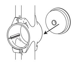
Install that end onto the Base by rotating it 1/4 turn counter clockwise until the Chopper Housing is vertical.
