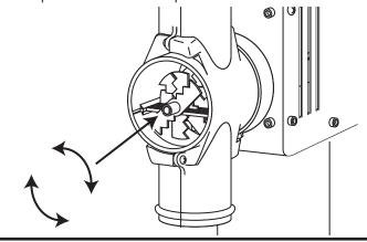
Install the remaining Shaft Bushing Housing into the opening of the Chopper Housing.
