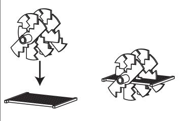
With the chopping edge of the blades facing to the left, slide the plate with the blades into the slots inside the
