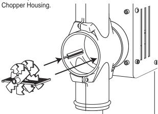
Slide the plate with the blades back onto the motor shaft of the base. Rotate the blades so that the blade shaft is installed onto the base motor shaft and is pushed back as far as possible.
