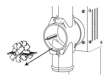
Remove the Chopper Housing by turning it clockwise 1/4 turn and pulling it out from the base.
