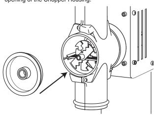
Install the End Cap onto the Chopper Housing by rotating it 1/4 turn counter clockwise to complete the
