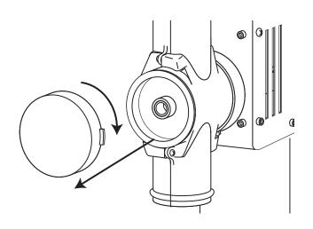
2 Remove the Shaft Bushing Housing.
