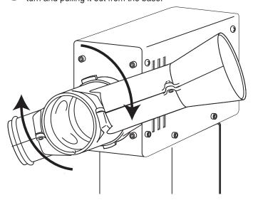
Remove the other Shaft Bushing Housing from the Chopper Housing.
