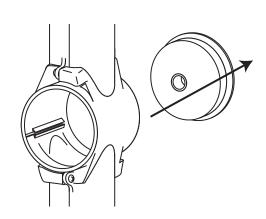
Clean the Chopper Housing, Blades, Shear Plate, Shaft Bushing Housing and End Cap using a brush and
