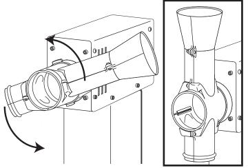
Place the Chopping Blades into the Shear Plate so that it is centered on the Plate.
