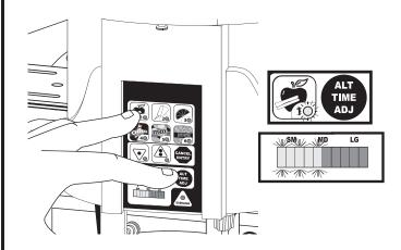
The number of lighted bars in the graph represent the length of time the serving is dispensed. Use the following chart to determine the bar graph setting needed for the desired serving size time.
