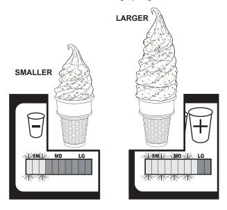
Repeat this process for each serving size (small, medium and large) until the correct serving time for each size is set.
