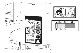
The number of lighted bars in the graph represent the length of time each layer is dispensed. Use the following chart to determine the bar graph setting needed for the desired dispense time for each ingredient layer.
