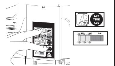
To increase the ingredient concentration (ie, add more ingredients to the serving), press the LARGE CUP (+) key. To decrease the concentration (ie, for less ingredients) press the SMALL CUP (-) key.
