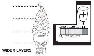
To decrease the timing (for more narrow layers), press the SMALL CUP (-) key until the correct number of bar graph lights are lit.
