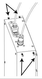
Remove the cable bushings from the splash guard slots.
