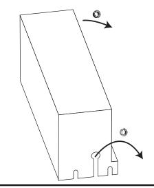
3 Pull apart each bushing and clip them around the power cord and the electronics box cord, with the lip of the bushing facing away from the electronics box connections.
