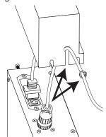
Snap each bushing into the slotted holes on the sides of the splash guard, with the lip on the outside.
