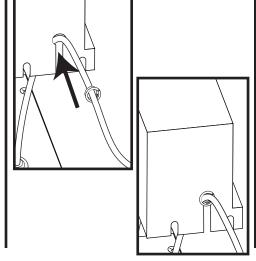
Slide the splash guard over the end of the electronics box and onto the loosened screws. Slide it forward as far as it will go. Tighten the four screws to secure the assembly.
