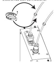
Slide each cable through the slotted holes of the splash guard, with the bushings to the outside. The cables should run from the electronics box, to the inside of the splash guard, and through the slotted holes to the outside of the splash guard.
