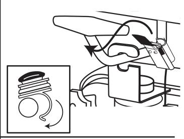
Slide the Spigot Switch Assembly toward the handle so that the Switch lever is depressed when the draw handle is grasped.
