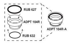
Install the two black o-rings onto the ADPT 104R as shown, and then install the ADPT 104R-A adapter onto the freezer spout.
