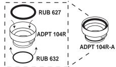
Install the two black o-rings onto the ADPT 104R as shown, and then install the ADPT 104R-A adapter onto the freezer spout.
