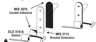
NOTE: MULTIPLE MOUNTING SOLUTIONS ARE POSSIBLE USING SOME OR ALL OF THE SWITCH MOUNTING ACCESSORIES LIKE THE EXAMPLE ABOVE. SEE THE ELE 510 INFORMATION SHEET.
