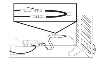
Insert the C tube through the hole with the black ring on the Cable Mounting Plate Assembly. Connect the tube to the C Valve inside of the freezer.
