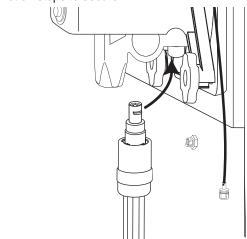
Connect the Cylinder Assembly line to the panel mount connector. Plug the switch extension into the stereo jack on the top of the housing assembly.
