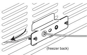
Angle the uppger bracket lip up through the 3rd vent slot from the bottom, so that the lower bracket lip can slide into the bottom vent slot. Slide the bracket down as far as it will go.
