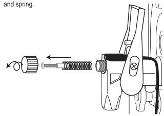
Remove the draw handle and the draw handle pin assembly from the modified door spout that came with the Flavor Burst FCB system.
