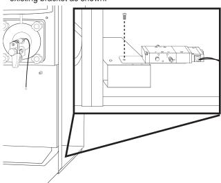
Connect the air tube to the B port on the valve. Use the tubing sleeves to secure the tube on the barb connection.
