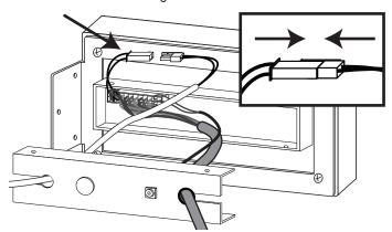
Reinstall the plate back onto the Touchscreen, securing it
