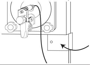
Remove the panel and drill the 7/16" hole where marked. Deburr the hole if necessary.
