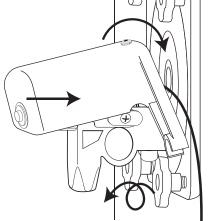
Insert the 9-Tube Assembly into the syrup port on the modified draw spout. Rotate the 9-Tube Assembly until motion stops to secure.
