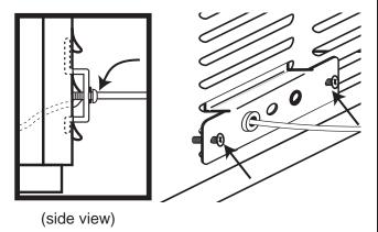
Connect the female spade connectors of the Rotor Cable D to the male connectors on the D Valve.
