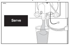
4. When the serving is nearly complete, release the "SERVE" key, but continue to hold the container under the spout to catch dripping product. The auto draw dispense mode is programmed to dispense a small amount of unflavored product at the end of the serving to help clear the spout and reduce carryover.
