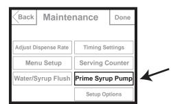
In the Prime Syrup Pump mode, press the first flavor key to prime the syrup line. The syrup flow will shut off automatically after 15 minutes. To cease flow earlier, press the flavor key again. Do this for all 8 flavors and
