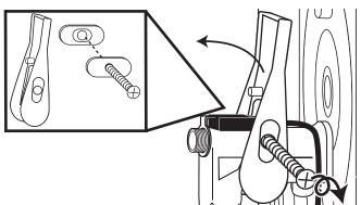
Disconnect and remove the spigot switch assembly. Ensure the two o-rings are in their respective grooves inside the syrup port.
