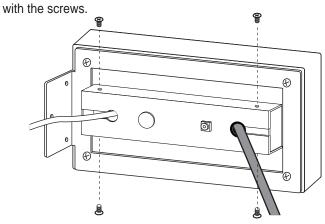
Gently pull any excess rotor cable through the hole. Snap the strain relief around the cable near the bracket plate.
