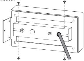
Carefully pull the plate away from the connections, without disconnecting any wires inside.
