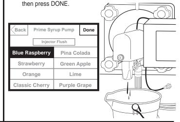
When the FCB product has frozen down, place a container under the spout. Draw a serving by selecting one or more flavors from the Touchscreen and press and hold the button to dispense. When the cup is nearly full, release the button. FCB product will continue to flow for a moment to clear the flavor from the spout to reduces flavor carryover to the next serving. Test out all 8 flavors to ensure everything is working properly.
