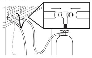
Open the valve on the CO2 tank and check for any leaks in the connections.
