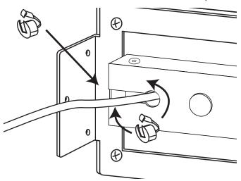
Insert the strain relief into the slotted hole to complete the rotor cable installation.
