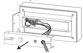
Remove the strain relief clamp from the slotted hole in the bracket plate.
