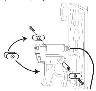
Insert the spring into the draw spout opening and install the cap onto the assembly.
