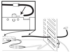
Ensure the CO2 tank is closed and then cut the supply line about 3" from the rear of the freezer. Install the Tee with the C tube in the CO2 supply line. Use clamps to seal the connections.
