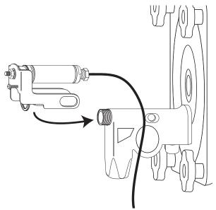
6 Install the draw handle pin assembly from the kit onto the Cylinder Assembly and tighten screw to secure.
