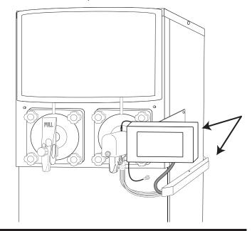
From the Touchscreen main menu, press the SETUP key in the upper left corner and enter the password if prompted (3141). If the SETUP key is not visible, press the top left corner anyway as it may be hidden if the self--serve mode is enabled.
