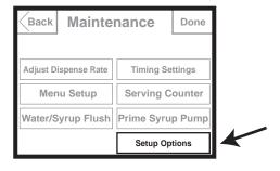
Ensure the "Enable FCB Purge" box is checked. If it is not checked, press on the box to check it. Also, ensure NONE of the other boxes are checked. Press to deselect any other checked boxes. Then press BACK.
