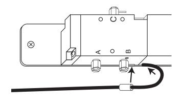
Install the cable mounting plate assembly on the same side as the Auto Draw Valve Assembly. Slide the spade connector ends of the cables through the 2nd slot from the bottom of the freezer's back vent cover.
