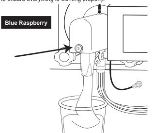
To adjust the product flow rate, remove the Housing from the Cylinder Assembly. Tighten the flow rate screw (clockwise) to decrease the product flow and increase flavor output. Loosen the screw (counter-clockwise) to increase the product flow and decrease flavor output. Return the Housing to the assembly.
