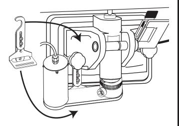
Using the adjustment screws, lengthen or shorten the bracket so that it supports the Injector Assembly in a level position. Also, install the Gear Box thumb nut onto the threaded post of the Gear Box. Tighten the screws and knob to complete the installation.
