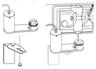
Position the Injector Assembly and Mounting Bracket so that they are horizontally level.
