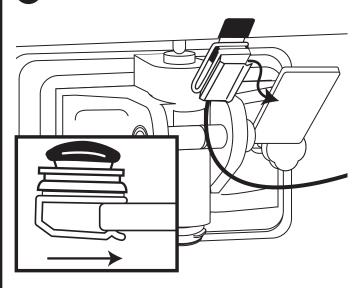
3 Slide the Switch Assembly toward the end of the draw handle so that the Switch lever is depressed when the draw handle is grasped.
