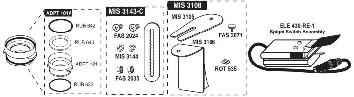
Assemble and install the Injector Adapter onto the freezer door spout. Ensure the o-rings and gasket are in their proper places.
