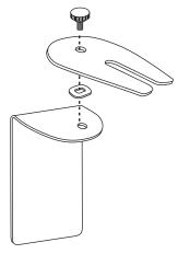
Attach the assembled MIS 3108 Mounting Bracket to the Injector System and then connect the Injector Head to the Injector Adapter.
