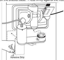
Reattach the Injector Head to the Adapter to complete the assembly and installation of the Mounting Bracket.
