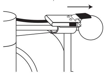
Be sure to fully engage the Spigot Switch jack to the Flavor Burst<sup>™</sup> keypad jack for normal operation. Do not neglect to check this connection during daily startup.
