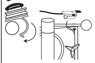
Position the Switch up towards the end of the draw-handle bar to complete switch installation.
