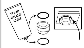
Install the RUB 625-O o-ring on the inside at the top of the adapter. Install the RUB 632 o-ring on the outside at the bottom of the adapter.
