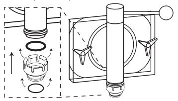
Position the Switch up towards the end of the draw-handle bar to complete switch installation.
