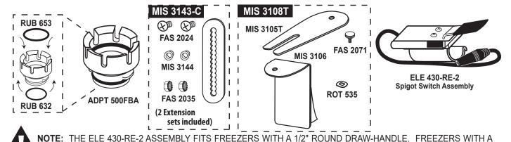
1/2" FLAT DRAW-HANDLE REQUIRE THE ELE 430-RE-1 SPIGOT SWITCH ASSEMBLY. Install and lube the RUB 653 O-Ring on the freezer door spout. Then, install the RUB 632 O-Ring on the Adapter
