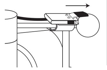
Rotate the Switch Assembly onto the draw-handle bar.
