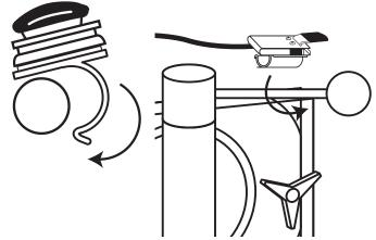
Be sure to fully engage the Spigot Switch jack to the Flavor Burst<sup>™</sup> keypad jack for normal operation. Do not neglect to check this connection during daily startup.
