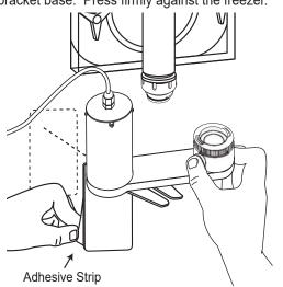
Reattach the Injector Head to the Adapter to complete the assembly and installation of the Mounting Bracket.
