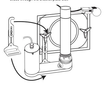
Using the adjustment screws, lengthen or shorten the bracket so that it supports the Injector Assembly in a level position. Also, install the Gear Box thumb nut onto the threaded post of the Gear Box. Tighten the screws and knob to complete the installation.
