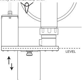
Move the bracket into position on the face of the freezer and ensure the Injector Assembly is level. On the freezer panel, mark around the bottom and sides of the bracket using a pencil.
