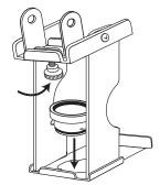
Remove the locking pin and the draw-handle from the freezer door.
