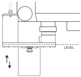
Move the bracket into position on the face of the freezer and ensure the Injector Assembly is level. On the freezer panel, mark around the bottom and sides of the bracket using a pencil.
