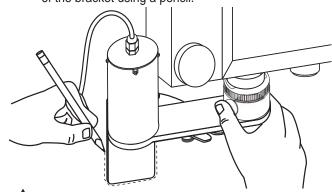
**NOTE:** BE SURE THE SURFACE OF THE FREEZER WHERE THE BRACKET BASE WILL BE ATTACHED IS THOROUGHLY CLEAN AND DRY.
