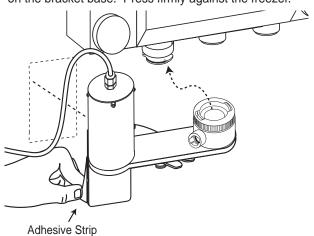
Reattach the Injector Head to the Adapter to complete the assembly and installation of the Mounting Bracket.
