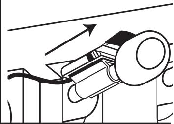
Be sure to fully engage the Spigot Switch jack to the Flavor Burst™ keypad jack for normal operation.
