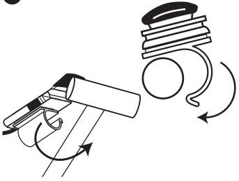
Position the Switch up towards the end of the draw-handle bar.
