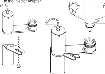
Position the Injector Assembly and Mounting Bracket so that they are horizontally level.
