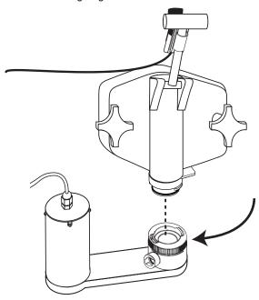
Hang the Suspension Bracket Assembly on the hand knob of the freezer nearest the Injector Assembly. Position the Bracket so that the bottom plate is underneath the Injector Assembly and the threaded post slides through the bracket plate slot.
