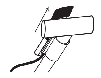
Be sure to fully engage the Spigot Switch jack to the Flavor Burst<sup>™</sup> keypad jack for normal operation.
