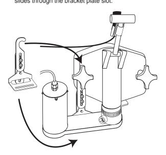
Using the adjustment screws, lengthen or shorten the bracket so that it supports the Injector Assembly in a level position. Also, install the Gear Box thumb nut onto the threaded post of the Gear Box. Tighten the screws and knob to complete the installation.
