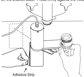
Reattach the Injector Head to the Adapter to complete the assembly and installation of the Mounting Bracket.
