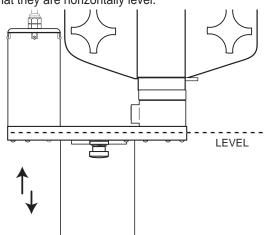
Move the bracket into position on the face of the freezer and ensure the Injector Assembly is level. On the freezer panel, mark around the bottom and sides of the bracket using a pencil.
