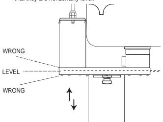
Move the bracket into position on the face of the freezer and ensure the Injector Assembly is level. On the freezer panel, mark around the bottom and sides of the bracket using a pencil.
