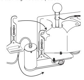
Using the adjustment screws, lengthen or shorten the bracket so that it supports the Injector Assembly in a level position. Tighten to secure.
