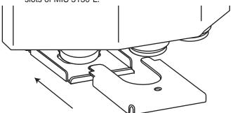
Thread the Hand Screw through the two bracket parts until snug to secure.
