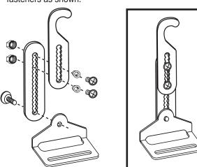
**NOTE:** IF MORE HEIGHT IS NEEDED, USE MULTIPLE EXTENSION BRACKET KITS WITH THE SUSPENSION BRACKET.
