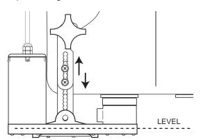
Install the Gear Box thumb nut onto the threaded post of the Gear Box and tighten to complete the installation.
