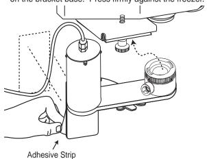
Reattach the Injector Head to the Adapter to complete the assembly and installation of the Mounting Bracket.
