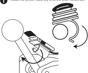
Position the Switch up towards the end of the draw-handle bar to complete the Installation.
