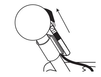
Be sure to fully engage the Spigot Switch jack to the Flavor Burst™ keypad jack for normal operation.
