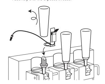
Replace the freezer handle and ensure that the Switch Assembly is the desired position as you secure the handle
