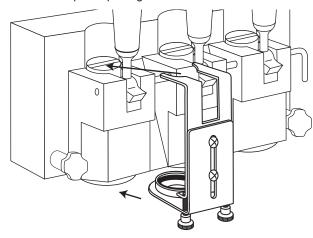
Tighten each hand screw firmly, then tighten each bracket screws to secure the assembly.
