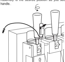
Be sure to fully engage the Spigot Switch jack to the keypad jack for normal operation.
