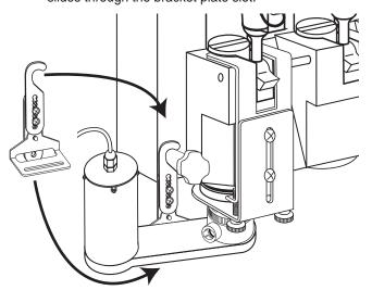
Using the adjustment screws, lengthen or shorten the bracket so that it supports the Injector Assembly in a level position. Also, install the Gear Box thumb nut onto the threaded post of the Gear Box. Tighten the screws and knob to complete the installation.
