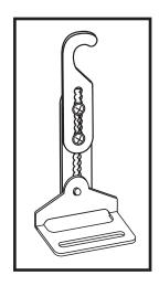
Attach the Injector Assembly to the spout adapter so that the Injector locking ring covers the adapter tabs. Turn the locking ring 1/4 of a turn to secure.
