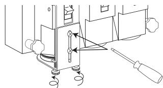
NOTE: BOTH BRACKET SCREWS SHOULD TIGHTEN FULLY AGAINST THE BRACKET ASSEMBLY, ALTHOUGH THE CORRESPONDING NUT WILL REMAIN LOOSE IN MOST INSTALLATIONS.
