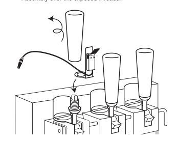
Replace the freezer handle and ensure that the Switch Assembly is the desired position as you secure the handle
