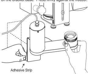
Reattach the Injector Head to the Adapter to complete the assembly and installation of the Mounting Bracket.
