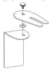
Attach the assembled MIS 3108 Mounting Bracket to the Injector System and then connect the Injector Head
