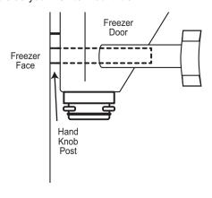
Right-Side Installation: Slide the Mounting Bracket through the gap until it touches the post, then slide the Mounting Bracket down and toward the freezer door spout until the hook rests on the post.
