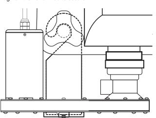
Rotate the locking collar off-center to secure the Injector Assembly to the Injector Adapter.
