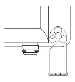
Left-Side Installation: Rotate the Mounting Bracket on its side as shown and slide the hooked end through the gap until it touches the post. Slide the Mounting Bracket up and away from the freezer door spout until the hooked end catches the post, and then allow the Bracket to rotate down to its normal hanging position.
