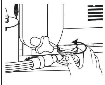
Attach the 9-Tube Assembly to the Injector Head. Rotate the 9-Tube Assembly off-center to lock and complete the installation.
