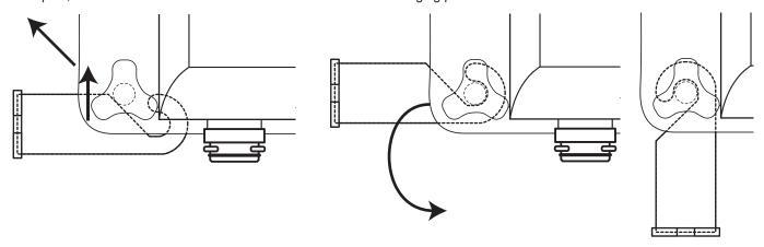
Attach the Injector Assembly to the Injector Adapter, slide the Injector Assembly onto the Mounting Bracket, and tighten the hand knob to secure.
