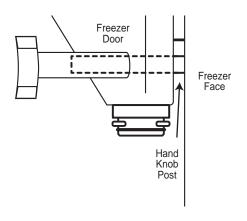
Right-Side Installation: Slide the Mounting Bracket through the gap until it touches the post, then slide the Mounting Bracket down and toward the freezer door spout until the hook rests on the post.
