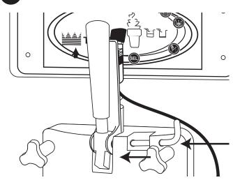
4 Connect the Switch to the keypad. Be sure to fully engage the jacks.
