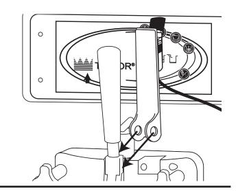
Replace the pivot pin to secure the assembly.
