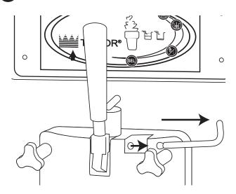
Mount the Draw Handle Switch over the draw handle so that the bracket holes line up with the pivot pin holes.
