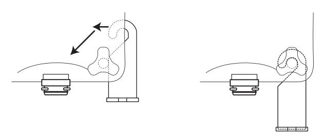
Left-Side Installation: Rotate the Mounting Bracket on its side as shown and slide the hooked end through the gap until it touches the post. Slide the Mounting Bracket up and away from the freezer door spout until the hooked end catches the post, and then allow the Bracket to rotate down to its normal hanging position.
