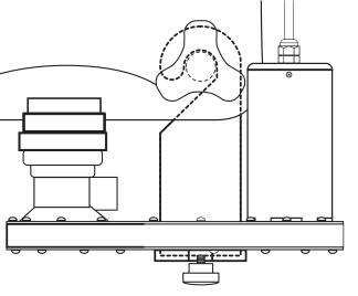
9 Rotate the locking collar off-center to secure the Injector Assembly to the Injector Adapter.
