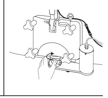
Attach the 9-Tube Assembly to the Injector Head. Rotate the 9-Tube Assembly off-center to lock and complete the installation.
