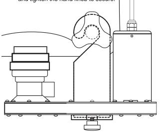
Rotate the locking collar off-center to secure the Injector Assembly to the Injector Adapter.
