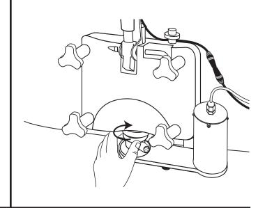
Attach the 9-Tube Assembly to the Injector Head. Rotate the 9-Tube Assembly off-center to lock and complete the installation.
