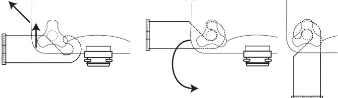
4 Attach the Injector Assembly to the Injector Adapter, slide the Injector Assembly onto the Mounting Bracket, and tighten the hand knob to secure.
