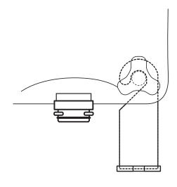
Left-Side Installation: Rotate the Mounting Bracket on its side as shown and slide the hooked end through the gap until it touches the post. Slide the Mounting Bracket up and away from the freezer door spout until the hooked end catches the post, and then allow the Bracket to rotate down to its normal hanging position.
