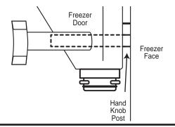
3A Right-Side Installation: Slide the Mounting Bracket through the gap until it touches the post, then slide the Mounting Bracket down and toward the freezer door spout until the hook rests on the post.
