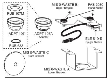
Lubricate the entire surface of the RUB 633 o-ring, ensure that the Adapter is properly assembled and lubricated, and then place the Adapter into the Lower Bracket.
