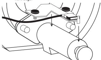
Place the Adapter and Lower Bracket over the spout opening, then tighten each hand knob evenly to secure the Upper and Lower Brackets.
