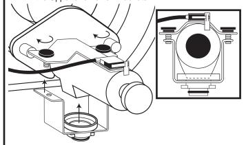
Unscrew and remove the draw handle knob and place the Front Bracket onto the threaded post. Then screw the draw handle knob back onto the threaded post and tighten to secure
