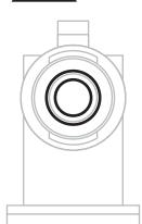
Press the MIS 3168 Restrictor Disk into the groove in the Blending Head inlet. This disk will reduce the flow of product by 1/3.
